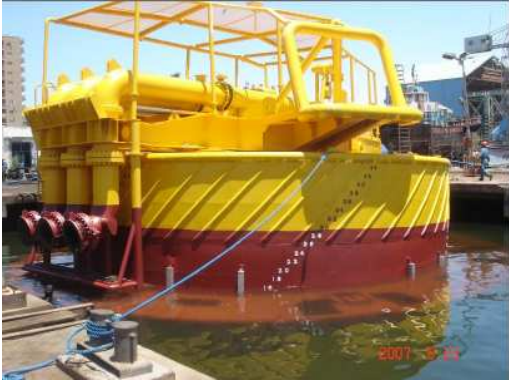
New build: Floating marine Service Boy Sumed, Ismailia El-Temsah yard Coating system Transozinc Epoxy Primer Transpoxy Barrier Transurethane Finish Transocean Cleanship
